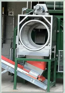
Trommel screen can be integrated into stationary exit end, providing automated screening of overs.
