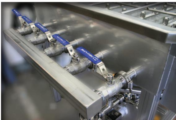
**Individual valve zone control for washing at less than full capacity.**
